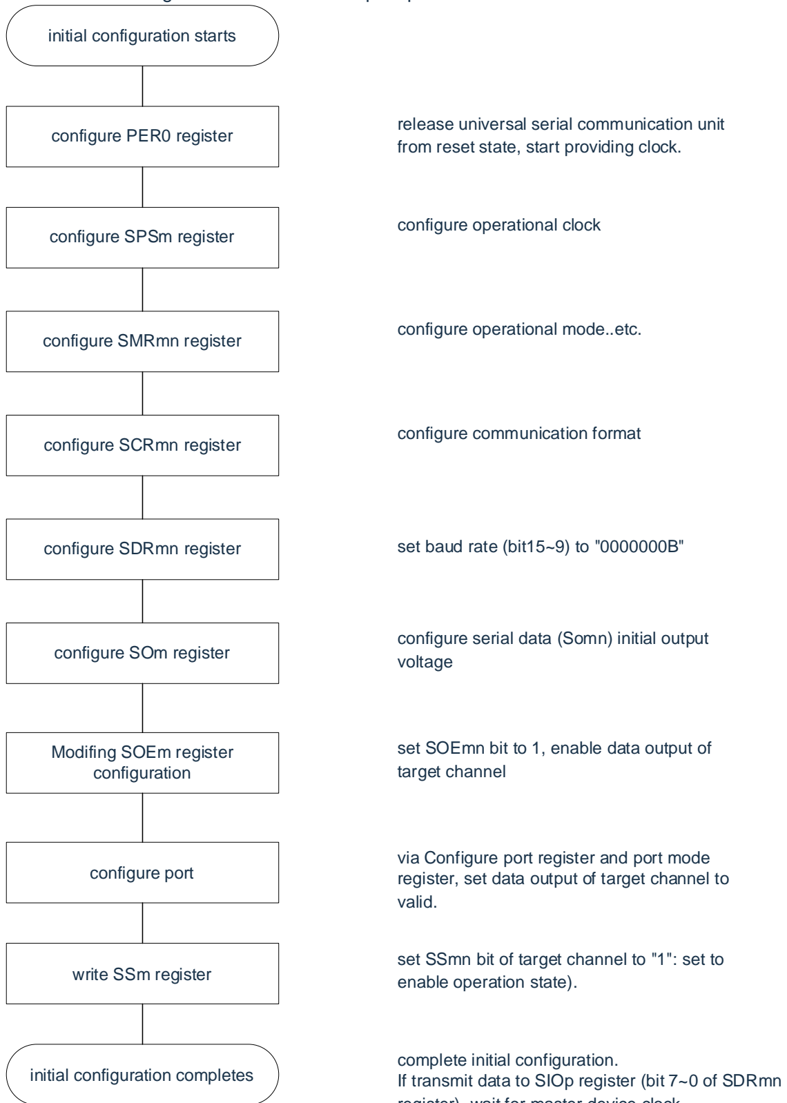
Figure 12-62 Initial setup steps for slave send and receive
